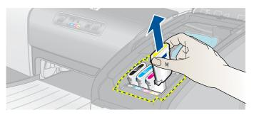
3 Insert the new ink cartridge into its own color-coded slot.
